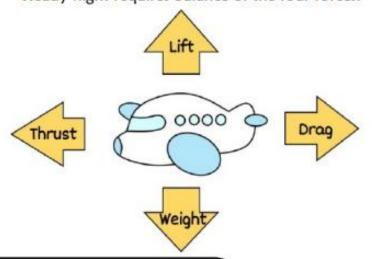
Thrust is the force that moves a flying machine in the direction of motion. It is created with a propeller, jet engine or rocket. Paper Aeroplanes get thrust from the person throwing it therefore to increase thrust, you'll need to throw harder!
